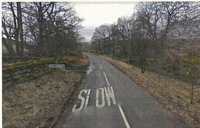
Photograph 1: C294 Carrshield southbound approach showing limited 'gateway' entry signing and markings
