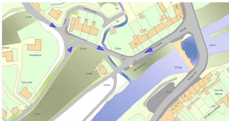
Figure 3 – location of gullies (red cross) and direction of flow in and around the war memorial
