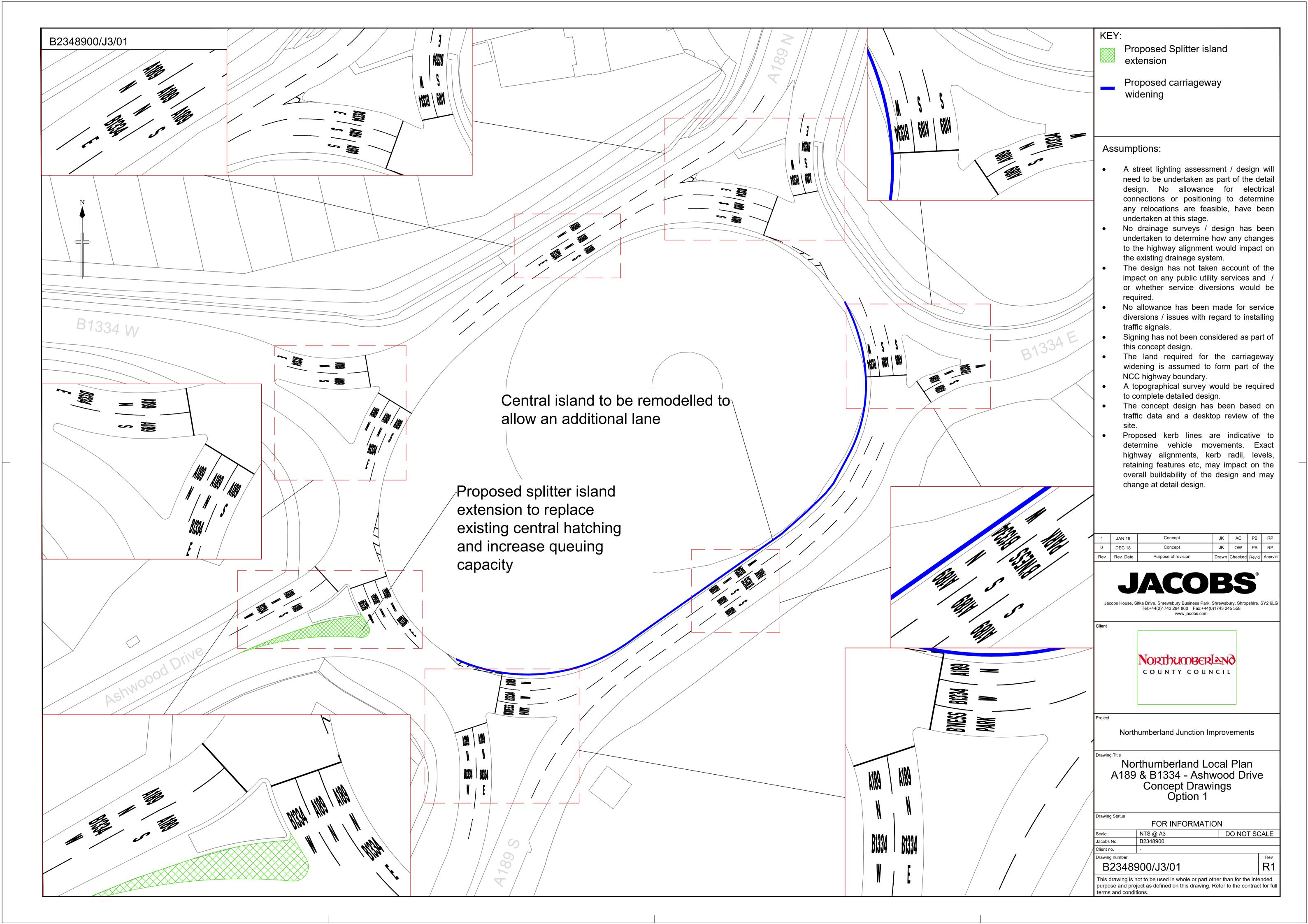
Proposed footway realignment to allow the installation of the roundabout
