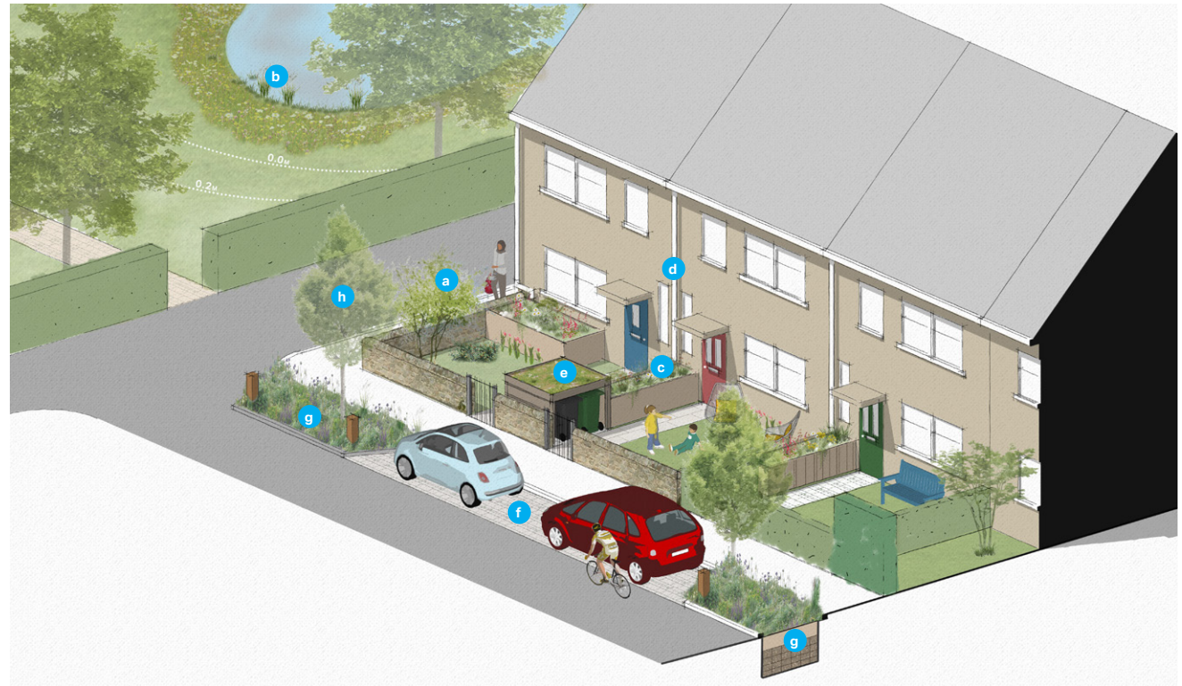
Figure 106: Illustration of selected typical SuDS features
