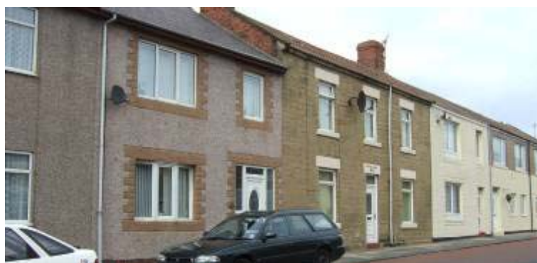
Later applied render can deaden the appearance of an area characterised by stone and brick, and harm the group value of terraces and building groups.
