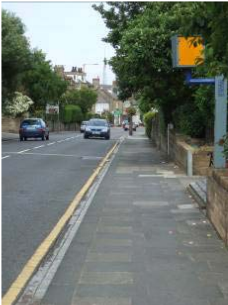
Black tarmac, concrete flags kerbs, scoria block gulleys (far right) and relatively unobtrusive road markings and speed camera.
