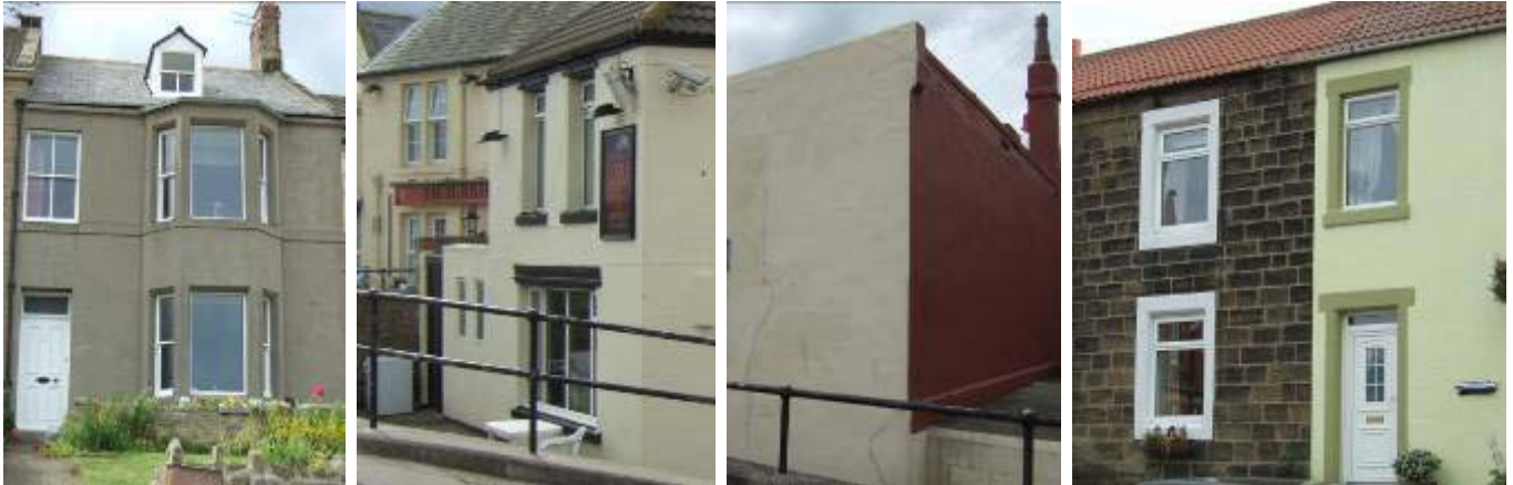
Render can flatten out architectural features. It is sometimes best left unpainted. Whitish tones seem artificial against richly textured sandstone. Modest use of pastel colours and muted, earthy tones can be suitable for this seaside location.
