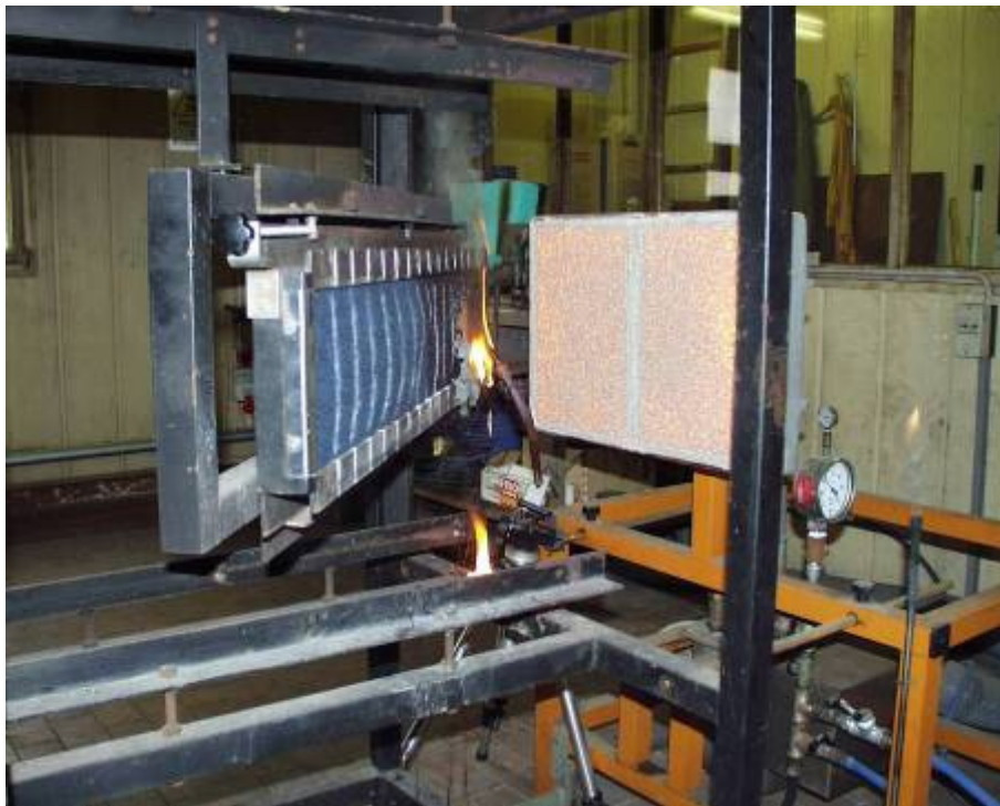
Figure 5.13 - UNI 9174:2008 Reaction to Fire of Materials Subject to Flame Ignition under Radiative Heat Exposition
