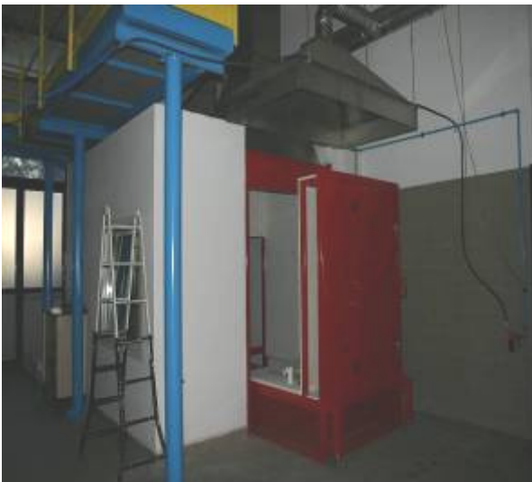
Figure 5.18 - UNI EN 13823 Single Burning Item (SBI) Equipment for Medium-Scale Tests on Construction Products
