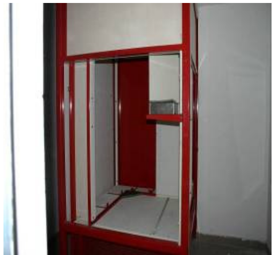
Figure 5.18 - UNI EN 13823 Single Burning Item (SBI) Equipment for Medium-Scale Tests on Construction Products
