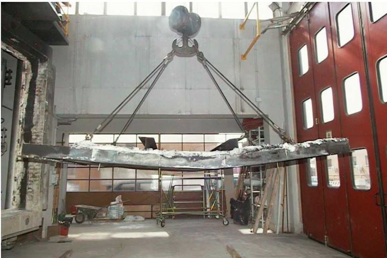
Figure 5.28 - Fire Resistant Floor Test – Side view after test
