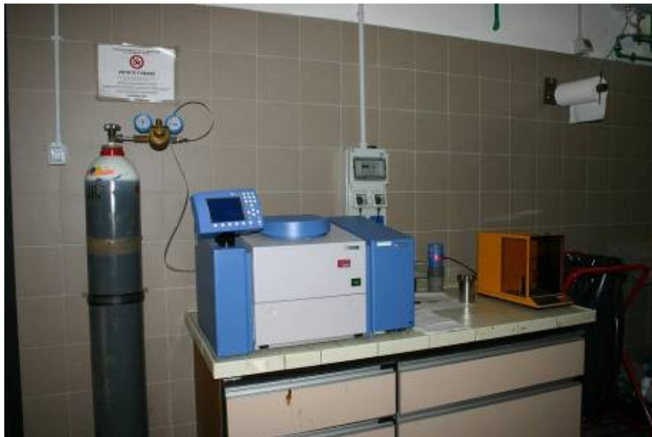
Figure 5.16 - EN ISO 1716 - Determination of the Heat of Combustion for Construction Products
