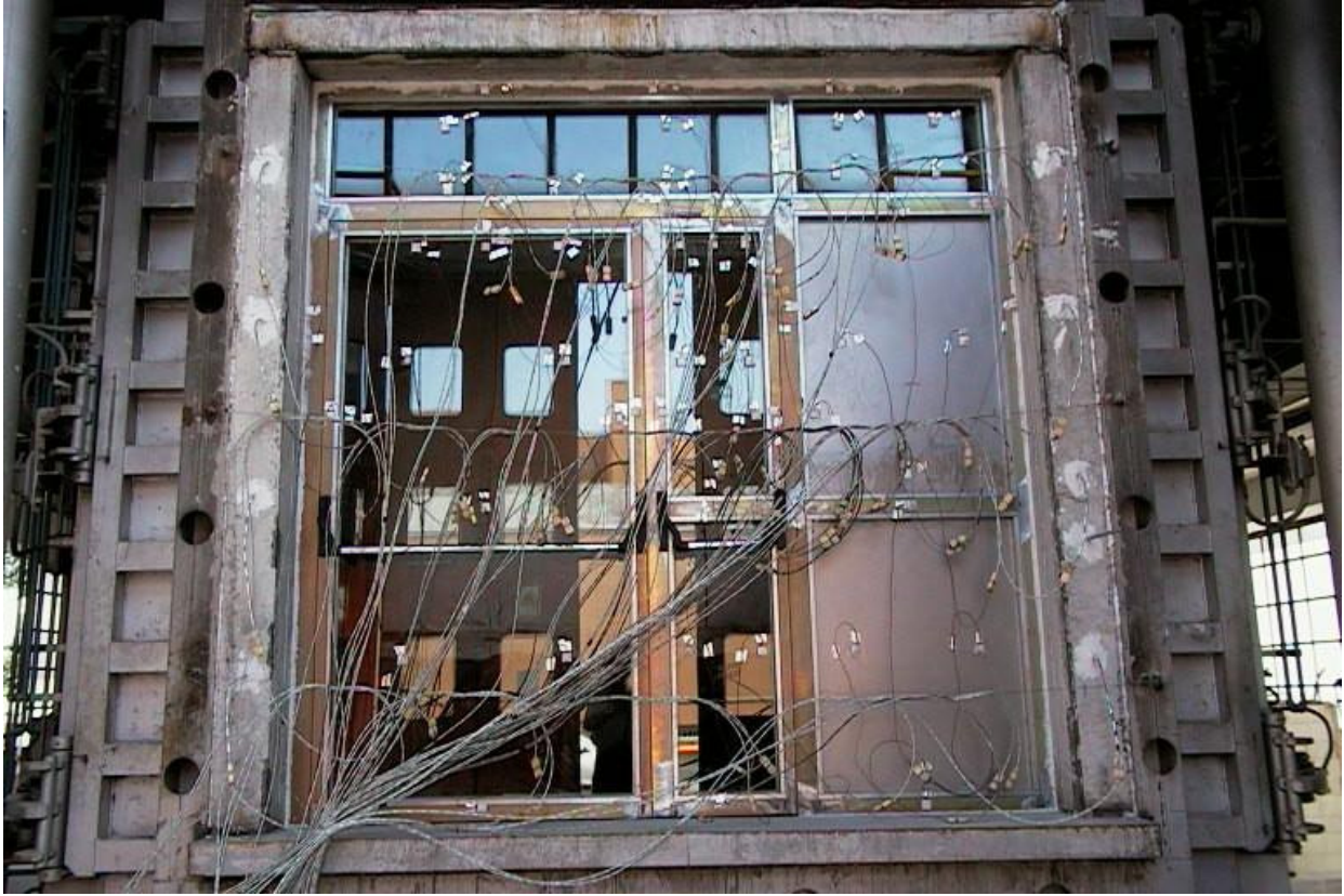
Figure 5.26 - Test on a Glazed Fire Door – exposed face after test
