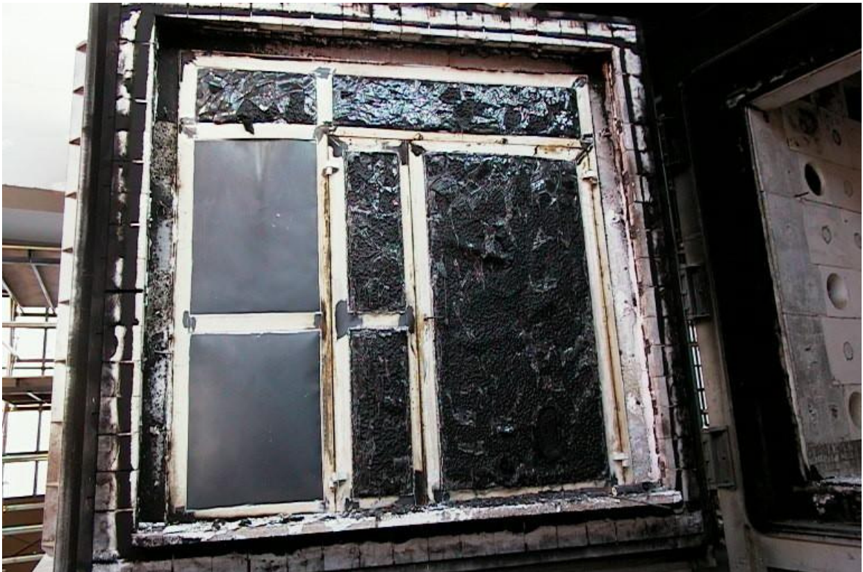
Figure 5.26 - Test on a Glazed Fire Door – exposed face after test
