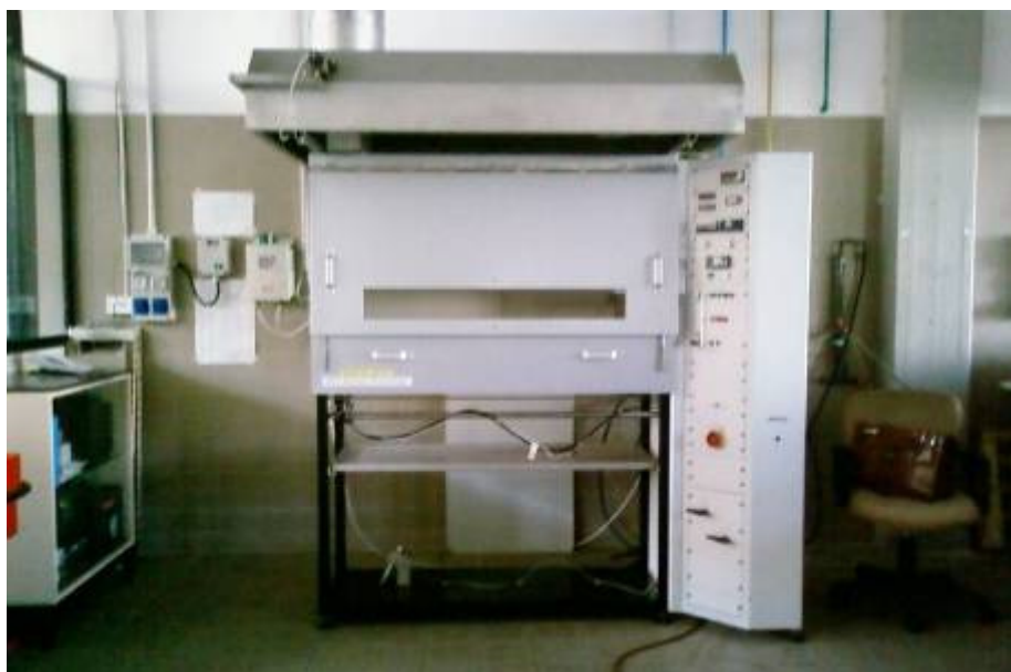
Figure 5.19 - UNI EN ISO 9239-1 Radiative Panel for Tests on Construction Products to be Installed at Floor
