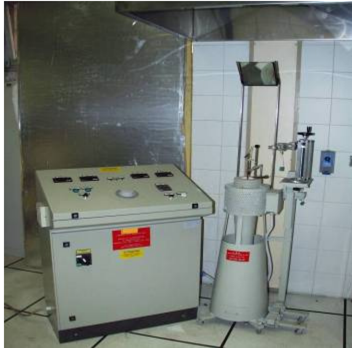
Figure 5.15 - UNI – ISO 1182 Non-Combustibility Test for Construction Products
