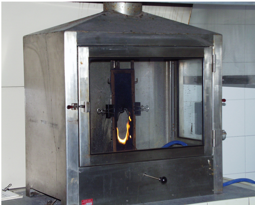
Figure 5.12 - UNI 8456/8457 – Combustible Materials Subject to Flame Exposition
