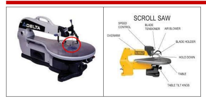
This machine has a spring steel 'sewing machine foot. It holds down the material and also prevents finger access. The gaps between the fingers of the guard allow the operator to see the cut line.
