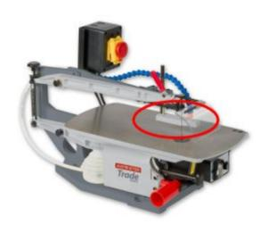
There is a replaceable teflon bung on the underside of the hold-down foot which is designed to press down on the top of the material while allowing free movement while cutting. The wire guard shown in front of the blade is sometimes replaced with a perspex guard on later models
