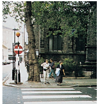
Street furniture and a well established tree obstructing the approach to a Zebra crossing.
