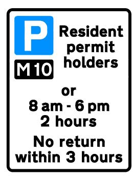
REPEATER SIGNS MOUNTED ON ALTERNATING LIGHTING COLUMNS WITHIN THE ZONE
