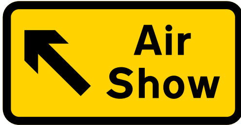
Example of an advance direction sign (ADS).
