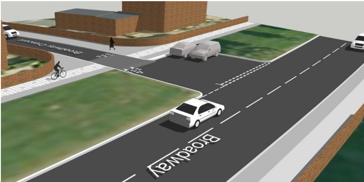
Figure 10: Raised table cycle and pedestrian priority crossing at Broadway Crescent.
