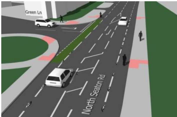
Figure 3: Light separation with reduced width central hatched area.
