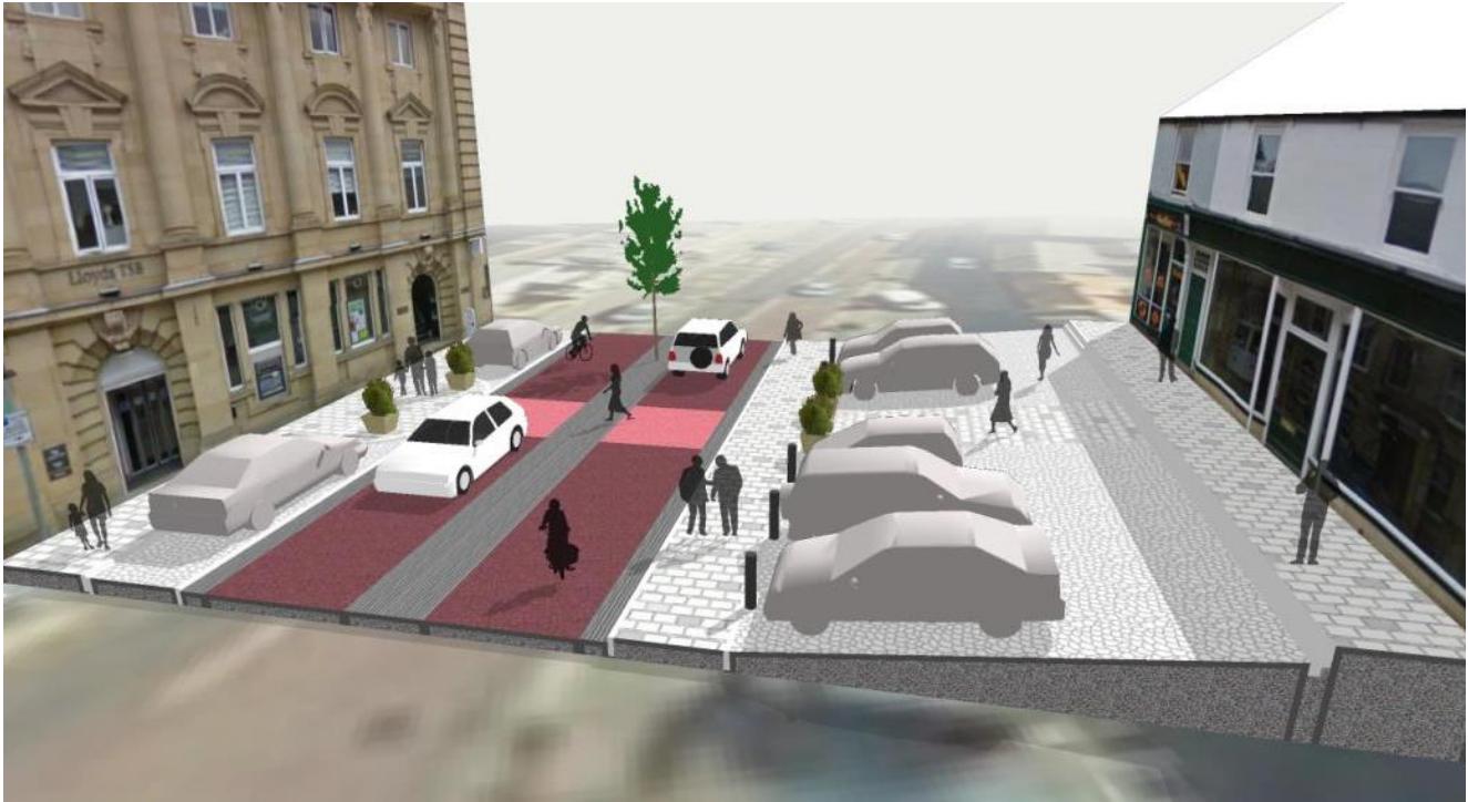
Figure 15: Visualisation of Market Street redesign with median strip and crossing points to break up car parking on and off the street.
