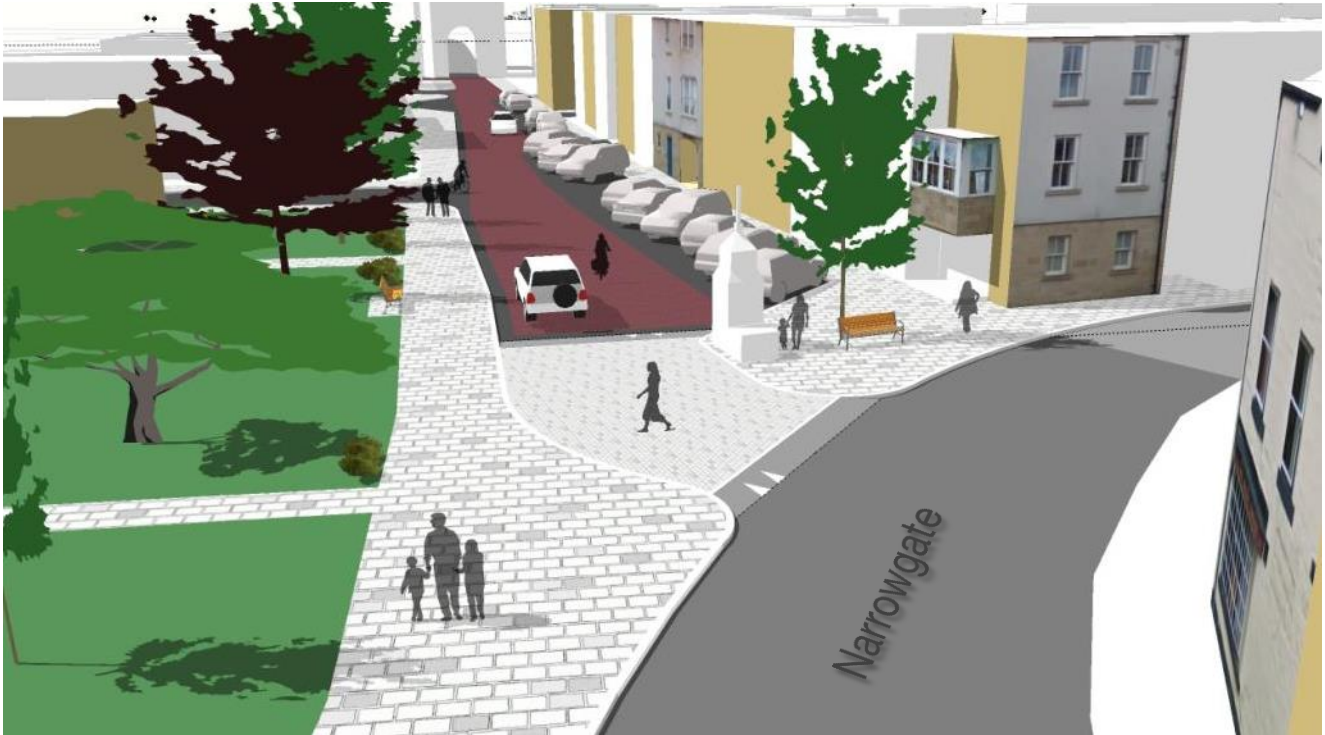
Figure 10: Pottergate (top: existing) and concepts (above) showing crossing improvements and an improved parking layout (circa 2 additional spaces)
