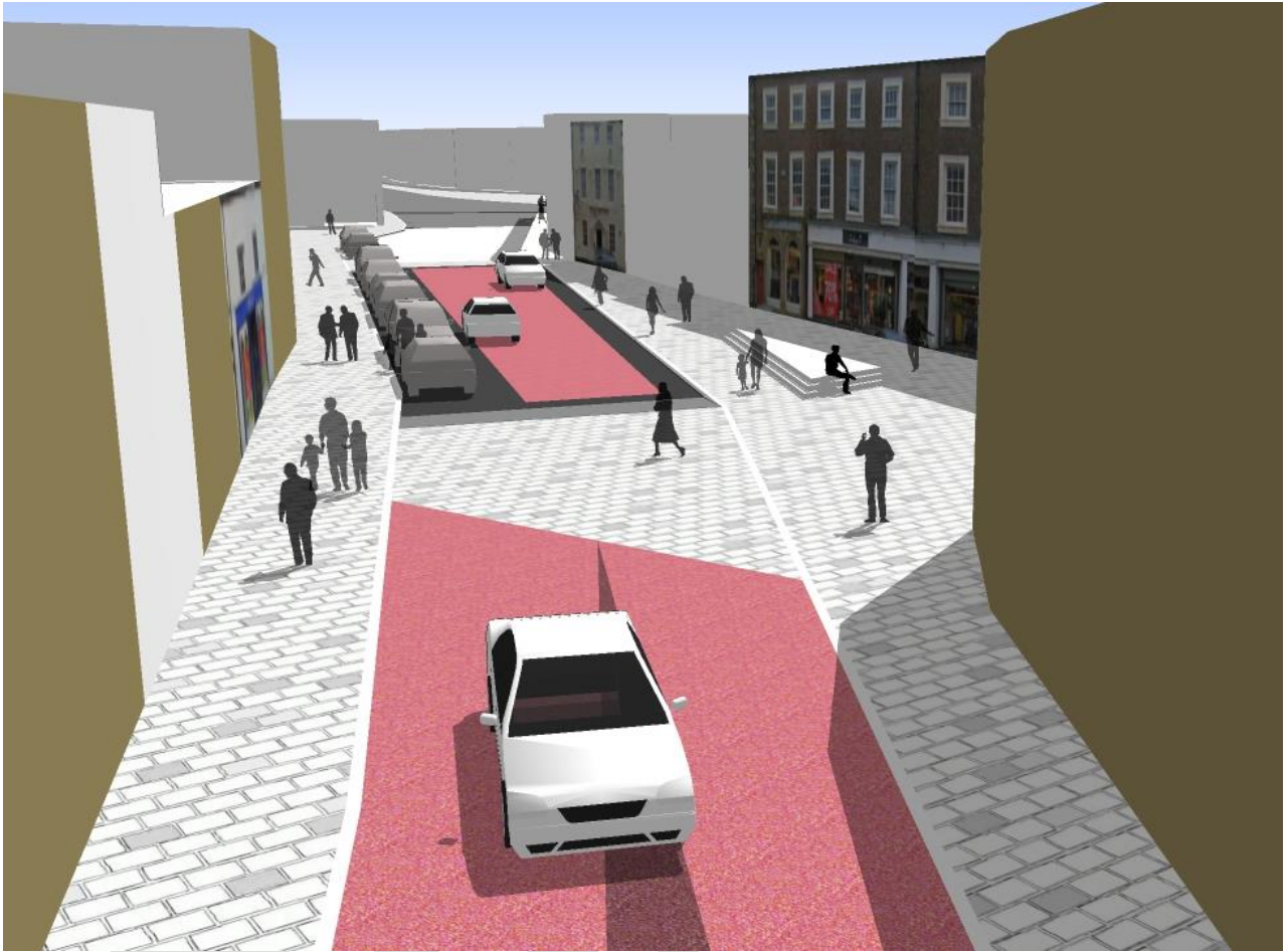
Figure 11: Narrowgate looking toward Bondgate Within with public space and crossing improvements. Restricting traffic from entering from the Narrowgate end and raising the surface of the road while maintaining a distinction between road and footway gives the perception of space on the street. More importantly, vehicles distanced from pedestrians at this pinch point. (Below: existing)
