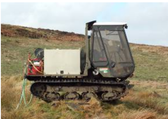
Figure 47 – Soft track vehicle with fogging unit
